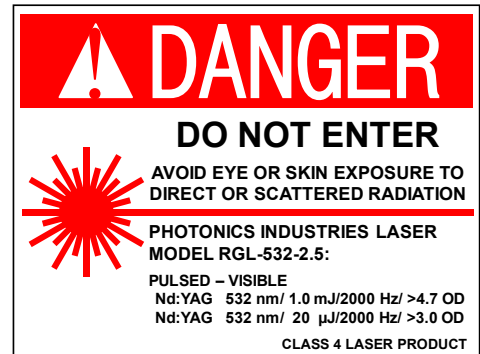
Figure 3-6: PI Laser Warning Sign
