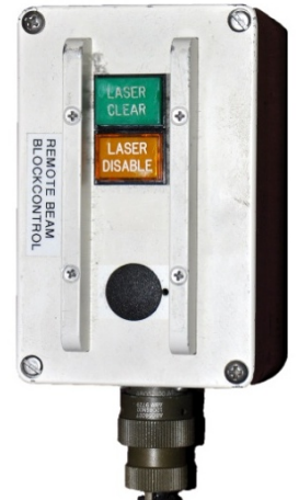
Figure 15: Remote Beam Block Control box
