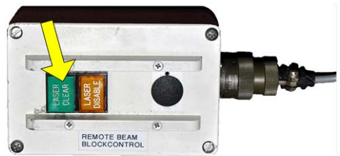
Figure 10: Remote Beam Block Control Box
