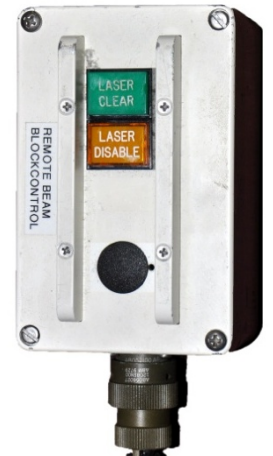
Figure 15: Remote Beam Block Control box
