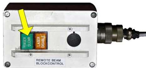
Figure 10: Remote Beam Block Control Box
